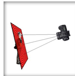
Now let's suppose you re-compose by tilting the camera downward. This not only changes the subject's position in the frame, it shifts the plane of focus; in this case, backwards. Although the plane of focus
